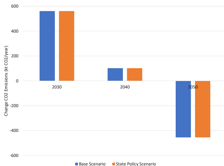
Figure 18. Change in the ammonia industry's net CO 2 emissions after electrification in Wyoming (Technical potential assuming a 100% adoption rate)
