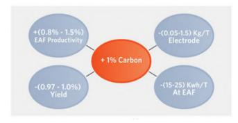
Figure 5: Effect of 1% carbon in DRI on EAF Operations (Sanjal, 2015)
