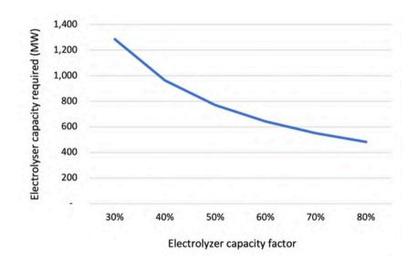
Figure 6: Electrolyzer capacity required to produce H<sub>2</sub> for 1 Mt/year steel with green H<sub>2</sub>-DRI process
